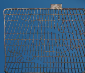
STANDARD GRID shown after 50,000 KM corrosion
